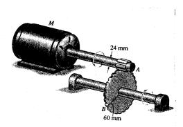
•16-5. The operation of reverse gear in an automotive transmission is shown. If the engine turns shaft A at  $\omega_A = 40 \text{ rad/s}$ , determine the angular velocity of the drive shaft,  $\omega_B$ . The radius of each gear is listed in the figure.
